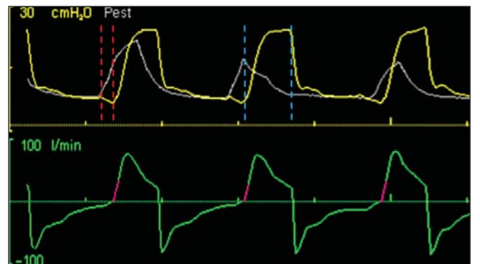
Figure 4 Screenshot from a Servo-I ventilator showing overlapping pressure curves; actual pressure curve in pressure support mode (yellow) and theoretical curve if patient were in NAVA mode (white). Inspiratory asynchrony (where neural inspiration begins before flow is triggered), is shown by lack of overlap of the red lines. Expiratory asynchrony (where neural demand starts to fall but the pressure trace shows that mechanical ventilation continues) is shown by lack of overlap of blue lines.
