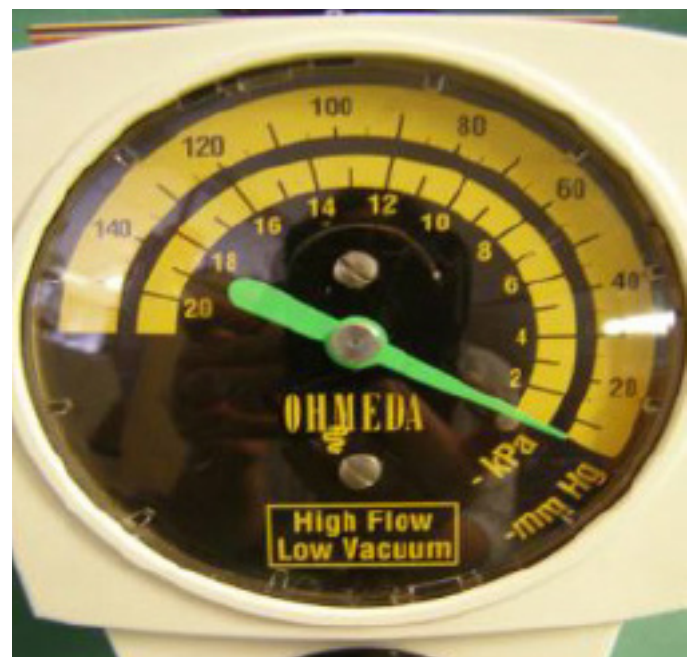
Figure 8: A low wall suction unit which displays both mmHg and Kpa.
